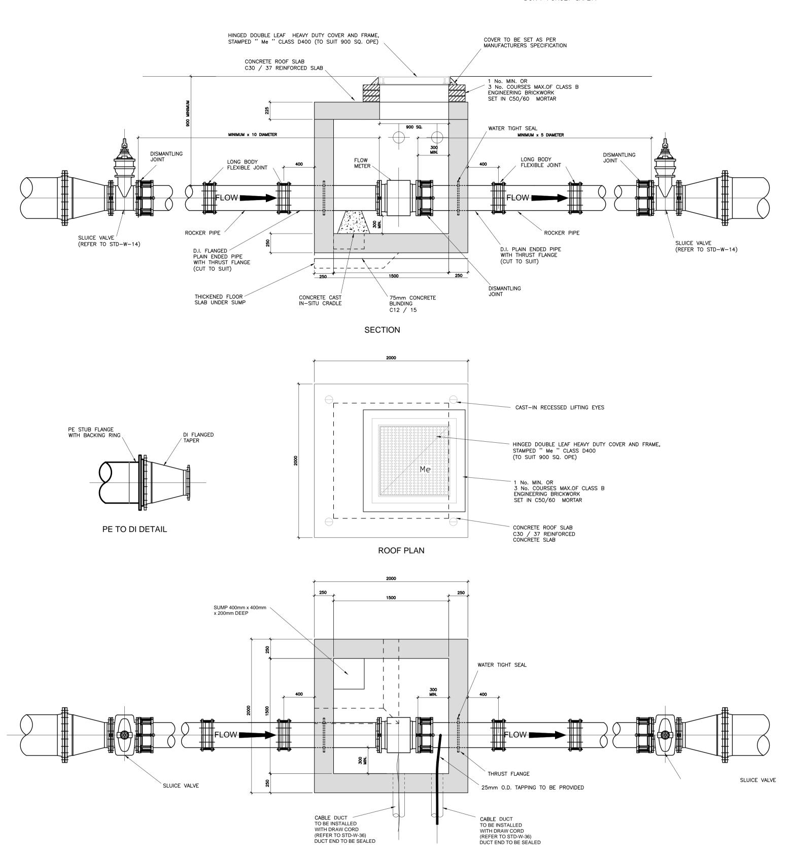
DETAILS OF WATERMETER CHAMBER
